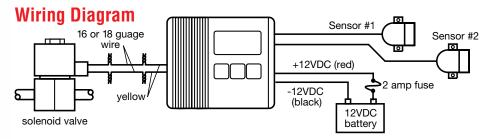
**Power requirements:** GS/6 with 1 sensor: 130mA; optional second sensor adds 85mA; when the solenoid is energized it adds 30mA.
